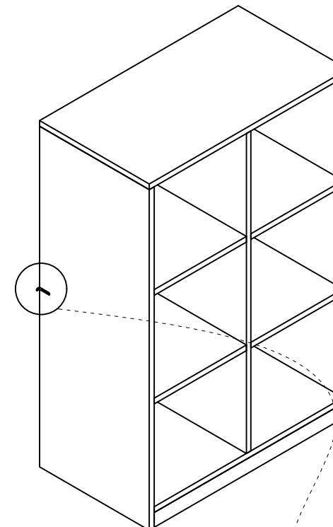
Connect the cabinet to the wall with self-tapping screws.
