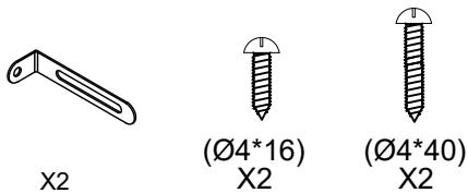
Connect the cabinet to the wall with self-tapping screws.
