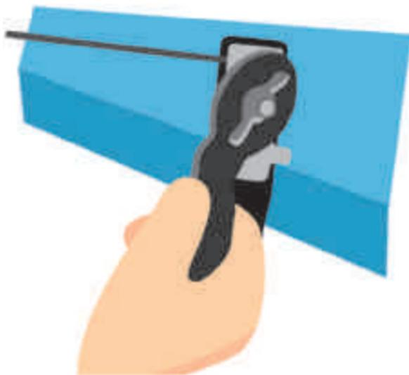
If it's too hard to do with bare fingers, Sammy can use the supplied spanner to tighten the wing screw.
