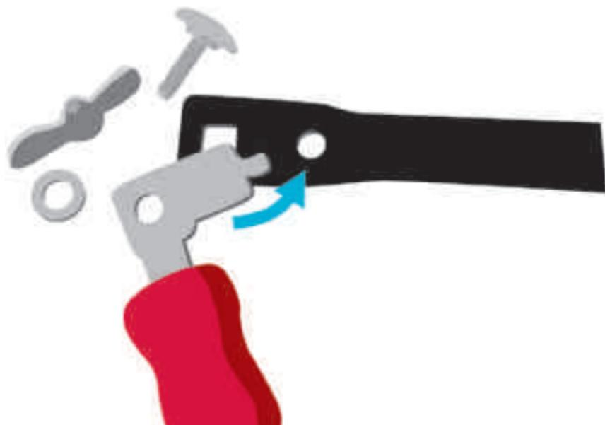
Here is the fretsaw – first step: screw the handle in its right position clamping it in the small hole. Now think of the blade.
